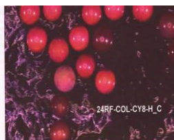
Figure 15. Resin in Hydrogen Form after Cycle 8 in 24° IX Column
